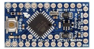
The Arduino Pro Mini is a microcontroller board based on the ATmega328.
