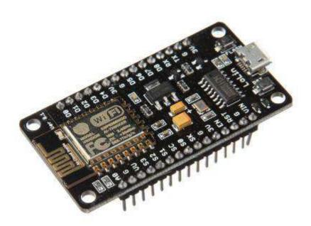
The NodeMcu is an open-source firmware and development kit that helps you to prototype your IoT product with few Lua script lines. The Development Kit based on ESP8266, integates GPIO, PWM, IIC, 1-Wire and ADC all in one board.
